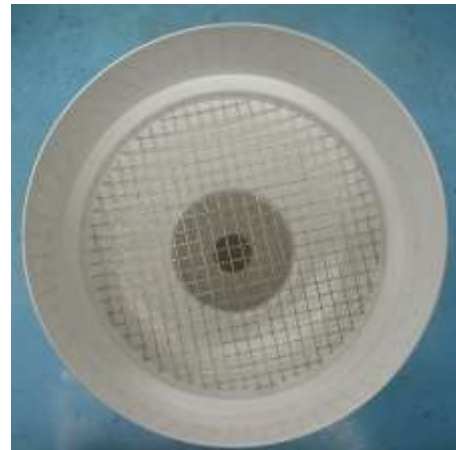
FIGURE 2.7: COLLECTION FUNNEL & ORIFICE SCREENS
