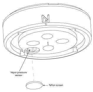
Figure 19 Vapor pressure sensor
