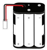
Figure 26 Battery polarity and pack orientation
