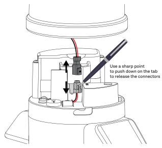
Figure 16 Disconnect pyranometer connector
