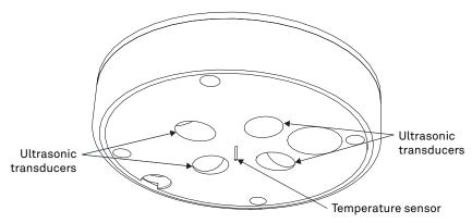
Figure 30 Temperature sensor and ultrasonic transducers
