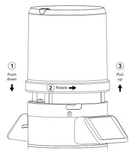
Figure 15 Removing ATMOS 41W rain funnel
