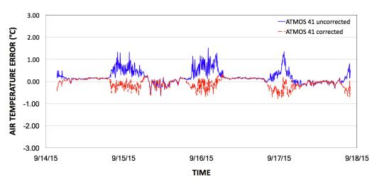
Figure 21 Corrected air temperature comparison with the aspirated radiation shield using 1-min measurement intervals
