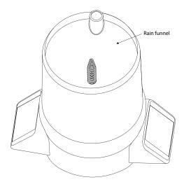
Figure 31 Rain funnel and pyranometer
