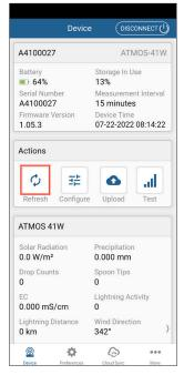
Figure 3 Information and current sensor readings
