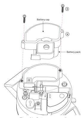
Figure 24 Battery cap removal
