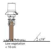
Add ATMOS 41W to ZENTRA Cloud (continued) If adhering to World Meteorological Organization (WMO)<sup>a</sup> siting standards, make sure the mount location has minimal slope and low vegetation height so the pyranometer found on top of the rain funnel will not be covered by shade.
