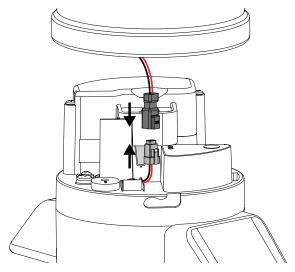
Figure 17 Pyranometer cable connector
