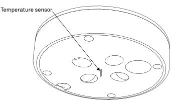
Figure 20 Temperature sensor
