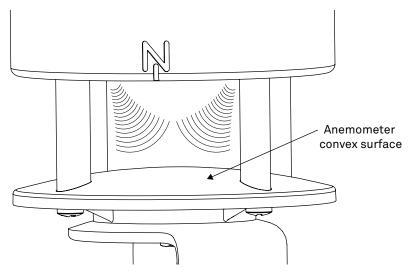
Figure 32 Convex base plate
