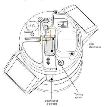
Figure 18 Downspout and screen
