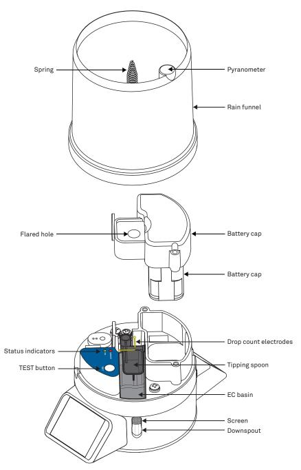
Figure 14 Rain funnel and rain gauge
