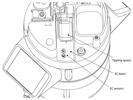
Figure 35 EC basin and EC sensor
