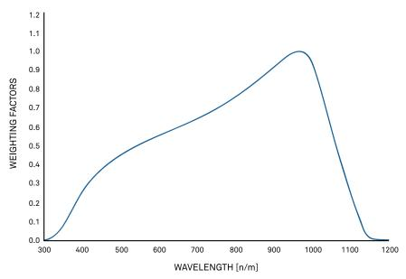
Figure 13 Spectral response estimate of Apogee silicon-cell pyranometers
