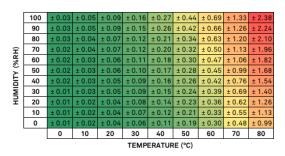
Figure 11 RH sensor accuracy
