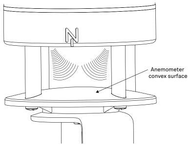
Figure 22 Anemometer
