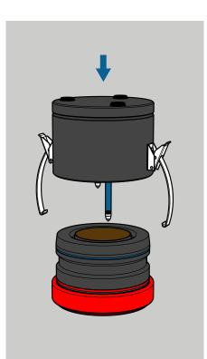
Put the refilled HYPROP<sup>®</sup> (for instructions about the preparation of the HYPROP<sup>®</sup> please read the HYPROP<sup>®</sup> manual) on top of the soil sample, turn the system upside down, remove the red sealing and close the HYPROP<sup>®</sup> clips.
