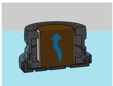
Fill the pan with water until it is just below the top of the sample ring (recommended times see below). Carefully tilt the sample including the saturation plate to let escape air bubbles.
