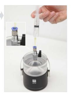
Screw 1, 2, 3 or 4 tensio shafts into the adapters.
