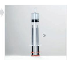
4 Push vacuum syringe bubble free onto the tensio shaft again.
