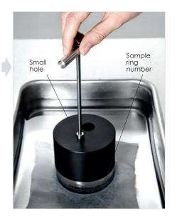
Fill drill holes with water to make sure air will not be pressed into the soil sample during assembly.
