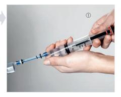
... until the plunger stoppers snap in. The vacuum in the syringe removes the air from the tensio shaft.
