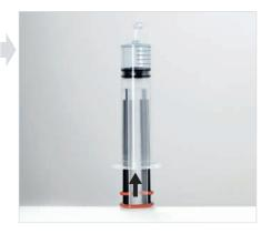
Push vacuum syringe filled with degassed water into the tube on the refilling attachment. Pull plunger until the plunger stoppers snap in. The pressure shown on the screen must reach a vacuum value equal to the atmospheric air pressure minus 20 hPa (2 kPa).
