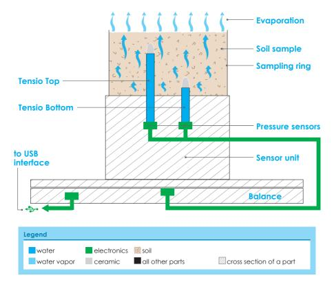
HYPROP 2 is a fully automated measuring and evaluation system based on Schindlers evaporation method (1980) to determine the hydraulic properties of soil samples. With tensiometers in two depths the device measures the soil water tension as well as the unsaturated hydraulic conductivity. Additional the volumetric water content is calculated through a continuous recording of weight loss.
