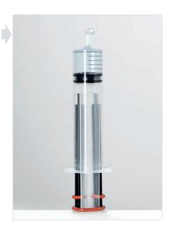
Degas water in the vacuum syringe analogous to degassing the reservoir syringe.
