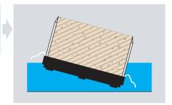
Put a plastic cap upside down on the sample ring. Do not fix it so that air can ventilate. The cap protects the soil from sun radiation and evaporation.
