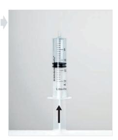
Push tube piece onto the tip of the syringe. Push plunger of the syringe until a meniscus builds up on the tube piece.
