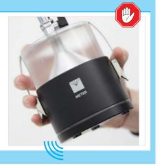
⑤ To relieve pressure hold plunger and syringe, press in the plunger stoppers and let the plunger slowly move forward.
