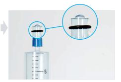
Push the ceramic of the first tensio shaft into the tube piece.
