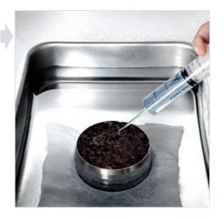
① Set the sensor unit cautiously upside down onto the soil sample. Make sure, no air gaps are generated and the soil is not compressed.
