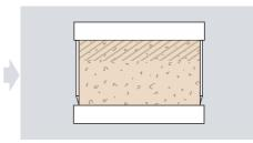
Turn soil sample upside down and put it on a table. Remove cap on top, place nonwoven cloth on the soil and put the filling bowl on the sample ring.
