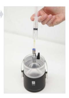
Fill vacuum syringe with 15 to 20 ml deionized water. Degas water in the syringe as explained on the previous pages.
