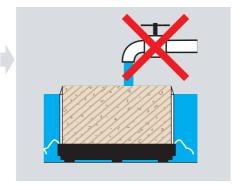
Let soil sample capillary saturate until the surface is shining.
