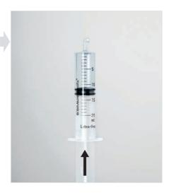
② Close reservoir syringe tightly with your finger, pull plunger completely and hold it.
