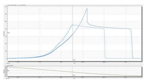
Site: Wolfenbüttel; soil type: slightly sandy loam. Ls3 (\$ 35%, U 48%, T 17%); measurements in winter 2011 at "Geoökologische Labormethoden 2011", TUBraunschweig. Evaporation: 2,75 mm/d, temperature: 21°C
