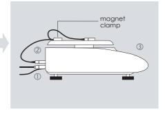
Connect the sensor unit and put it on the balance.
