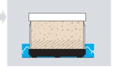
Raise the water level up to 5 mm below the sample rim (recommended times see below). Do not pour water on the sample – you may trap air. Use the time table below as a reference to determine how long samples take to saturate.
