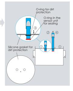
(5) Fill the silicone tubes immediately with deionized water.
