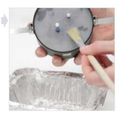
Clean also sample ring and silicone gasket above the bowl to avoid losses.
