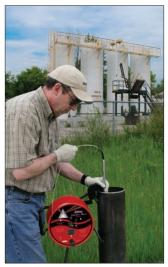
the probe enters a liquid the beam is refracted away from the detector which activates an audible tone and light.
